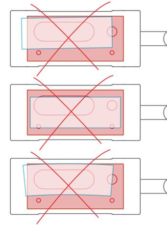
If there are air pockets between the protective film and the glass window after the film has been applied, do not attempt to remove them. Remove the protective film and start again with a new protective film as per the section *Preparation*.
